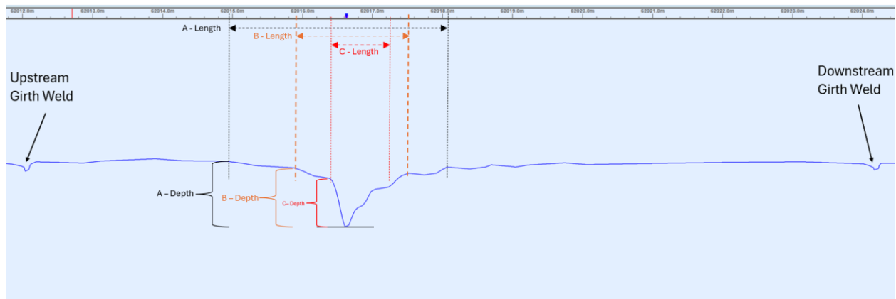
Figure 3: Axial View of Target Dent with Variable Stated Lengths and Depths on a Caliper Channel
